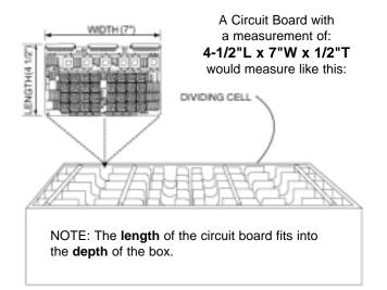
In measuring a circuit board, you must be aware of any components or leads that extend past the board. These extended parts could be damaged if loaded into the cell and placed at the bottom of the In-Plant Handler. Therefore, make sure that the width dimension has no protrusions. If your board has protrusions, then reverse the length and width dimensions to make sure your board fits properly in the In-Plant Handler. When in doubt, send us a sample of your circuit board.
