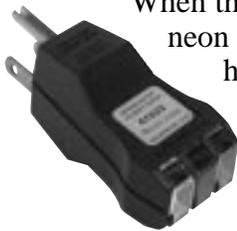
When the 41333 is plugged into an outlet, three neon lights on the unit indicate wiring of the hot, neutral, and ground lines. The sequences of the three lights indicate whether or not the outlet is wired properly. The unit also incorporates a banana jack that will accept a standard ESD Systems plug, allowing for grounding of an operator through the unit. Request Tech Brief PS-2044 for more information.
