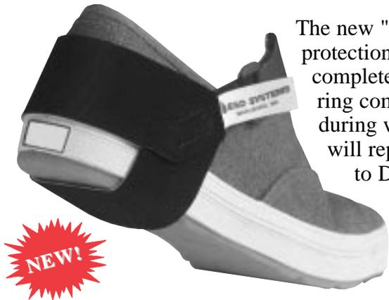
The new "Lifetime" foot grounder provides effective and economical ESD protection. Made from cross-linked tire grade rubber, the heel cup ensures complete charge dissipation and provides two wear surfaces. An elastic D-ring comfort system provides maximum ankle comfort by allowing for flex during walking. If this grounder ever wears out, simply return it and we will replace it FREE. Call customer service for complete details. Refer to Drawing 24500. Phone: (508) 485-7390 Fax: (800) 805-5665.
